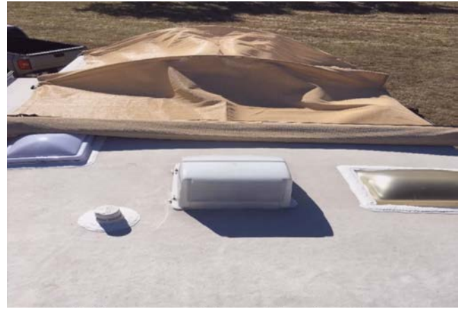
14) Pull cross strap until velcro pieces are aligned to arch the fiberglass rod. Attach velcro pieces together.
