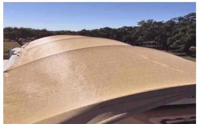
18) Once in back pull the canopy tight. Attach back straps. REFER TO STEPS 8-10.
