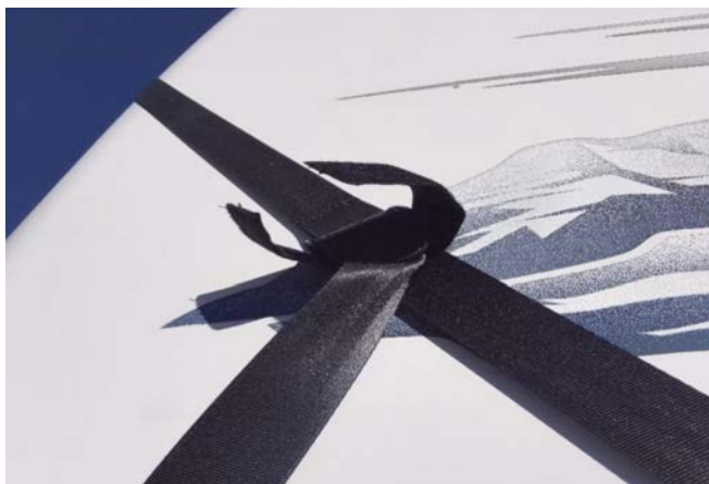
29) Install Velcro under buckle to protect RV.
