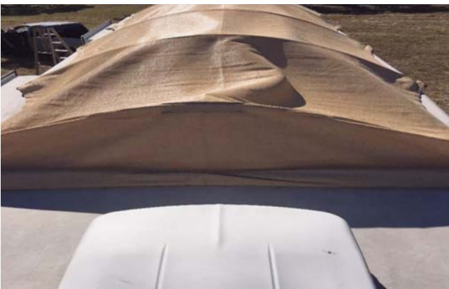
17) Repeat STEPS 11-16 until the canopy is fully unrolled (with arches) to the back of the RV.
