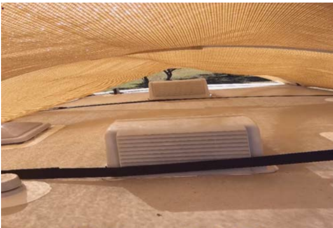
15) Try to avoid roof units. It is suggested to put cross straps towards backside of roof units, or in the direction needed to tighten the canopy.
