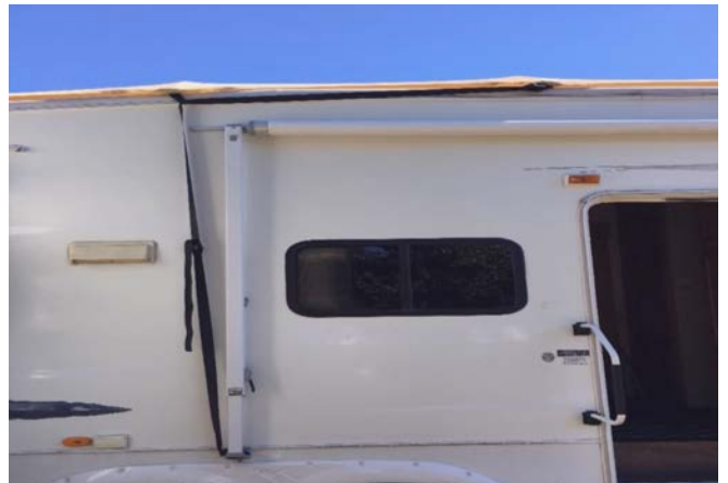
28) In this application, we used a 12' strap on top and 6' on bottom to avoid the awning.
