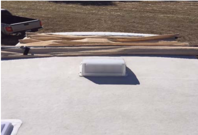
13) Continue to unroll canopy towards the back of the RV until the next cross strap is reached. USE CAUTION TO AVOID DAMAGE TO ROOF UNITS
