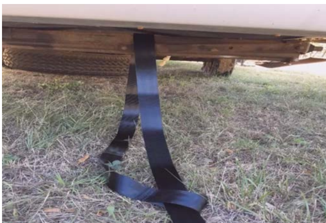
5) Attach (1) 12' strap to RV frame, ladder, hitch or bumper. Repeat with another 12' strap.
